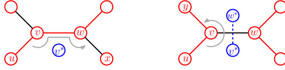
Fig. 2. Left: If we process an edge (v, w) in T , then we move to w in our traversal of T and the next edge, (w, x) in this case, is also incident to the vertex v^* we are visiting in our traversal of T^* . Right: If (v, w) is not in T , then in T^* we move from v^* to the vertex w^* corresponding to the face on the opposite side of (v, w) in G . The next edge, (v, y) in this case, is also incident to w^* .
