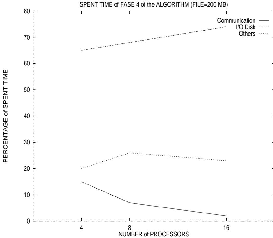
**Fig. 6.** Percentage of time spent in step 4 of the algorithm (which includes communication, I/O operations on disk, compression of suffix arrays, packaging of data to be transmitted, contention in suffix array transmission), considering a file of 200 MB.
