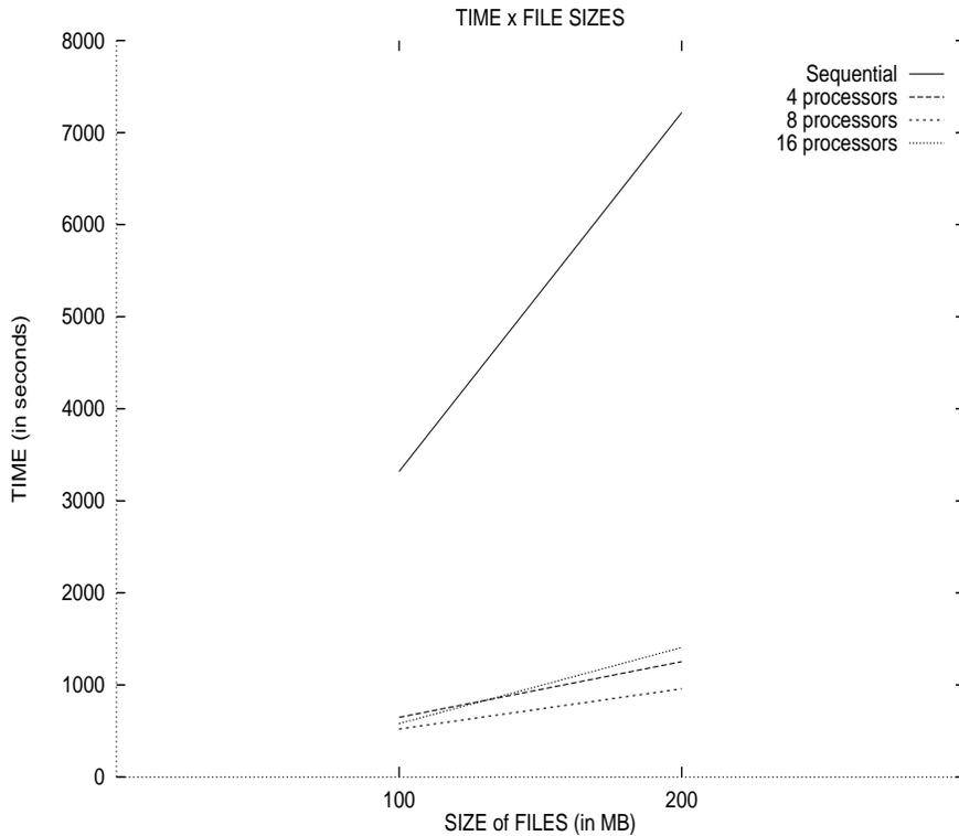
**Fig. 3.** Measures of elapsed time for index generation using 1, 4, 8 and 16 processors, connected by fast network at CENAPAD - MG/CO, considering files of different sizes.
