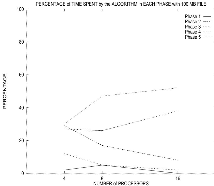
**Fig. 1.** Percentage of time spent by each step of the program, when it was submitted to a network of workstations in CENAPAD - MG/CO with a text input file of 100 MB.
