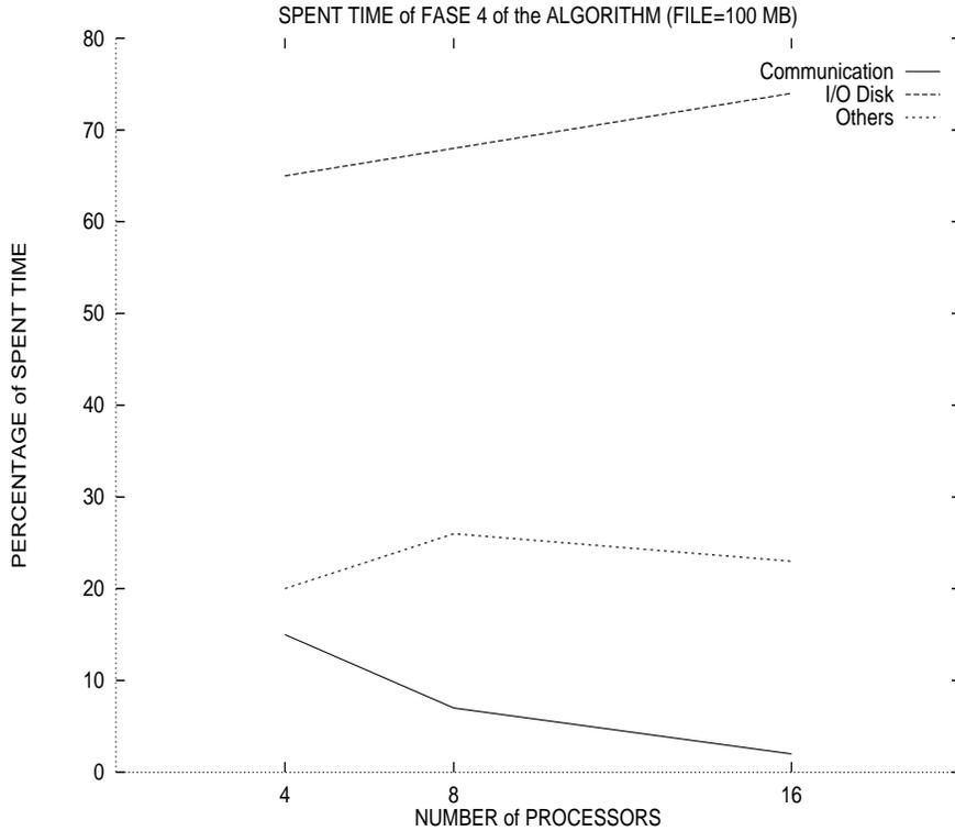
**Fig. 5.** Percentage of time spent in step 4 of the algorithm (which includes communication, I/O operations on disk, compression of suffix arrays, packaging of data to be transmitted, contention in suffix array transmission), considering a file of 100 MB.
