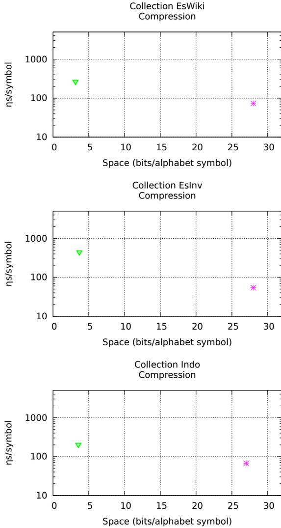
Fig. 4. Code representation size versus compression time for table based representations (TABLE, TABLE<sub>S</sub>, and TABLE<sub>E</sub>) and ours (COMPR). Time (in logscale) is measured in nanoseconds per symbol.
