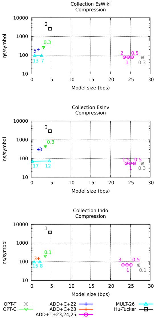
Fig. 8. Space/time performance of the approximate and exact approaches on compression. Times are in nanoseconds per symbol and in logscale. The numbers around the points are their redundancy as a percentage of the entropy.
