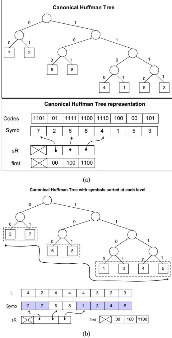
Fig. 1. An arbitrary canonical prefix code (a) and the result of sorting the source symbols at each level (b).
