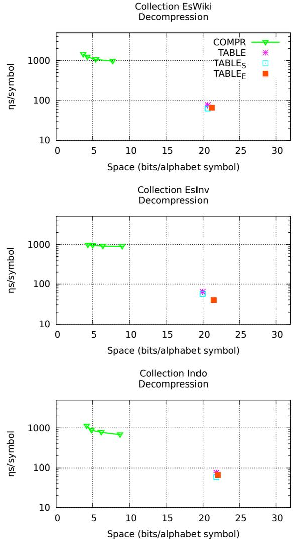
Fig. 5. Code representation size versus decompression time for table based representations (TABLE, TABLE<sub>S</sub>, and TABLE<sub>E</sub>) and ours (COMPR). Time (in logscale) is measured in nanoseconds per symbol.
