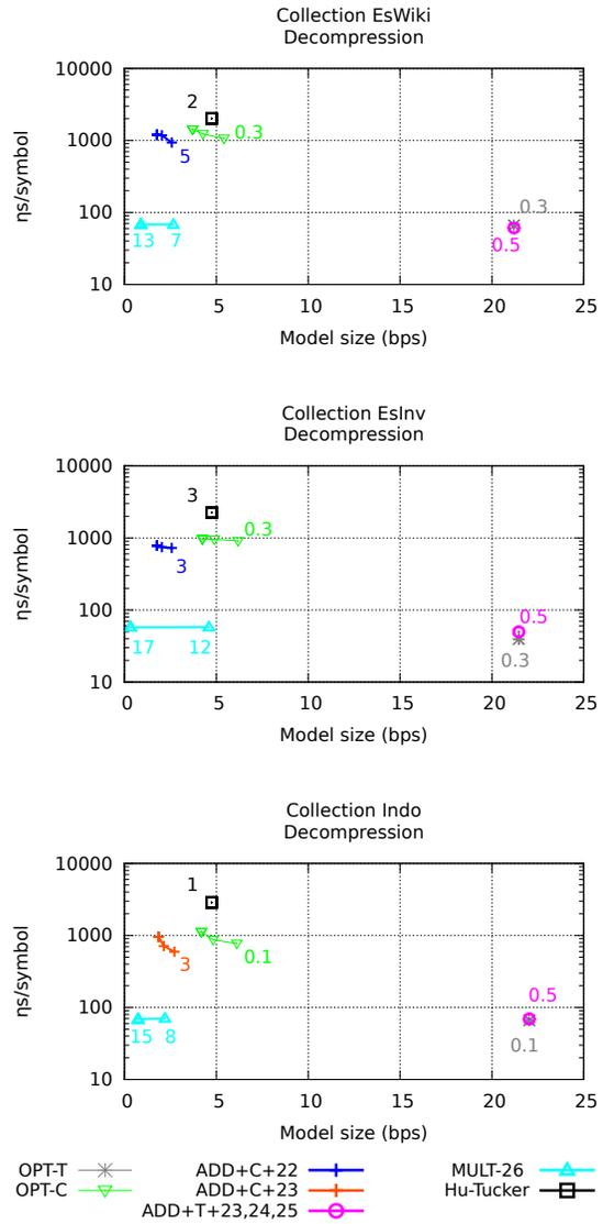
Fig. 9. Space/time performance of the approximate and exact approaches on decompression. Times are in nanoseconds per symbol and in logscale. The numbers around the points are their redundancy as a percentage of the entropy.
