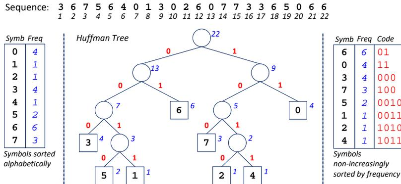
Figure 1: An example of Huffman coding. A sequence of symbols on top, the symbol frequencies on the left, the Huffman tree  $\mathcal{B}$  in the center, and the corresponding codewords on the right. The blue numbers on the tree nodes show the total frequencies in the subtrees. The sequence uses  $n \lg \sigma = 66$  bits in plain form, but 61 bits in Huffman-compressed form.
