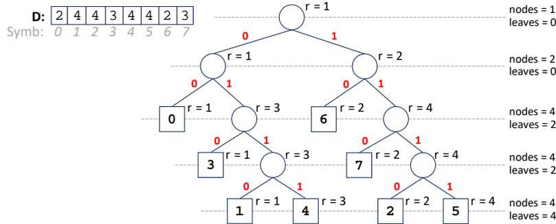
Figure 7: Our representation for the tree of Figure 4. We only store the sequence  $D$  and the values  $\text{nodes}$  and  $\text{leaves}$  at each level. For each node  $v$  we show its  $r_v$  value.
