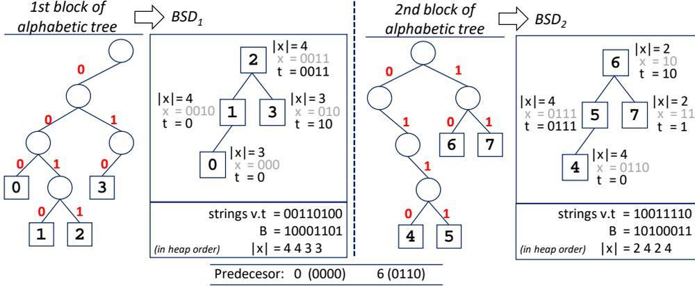
Figure 5: Our representation of the code for wavelet matrices of Figure 4. For each BSD structure we only store the concatenated strings  $v.t$ , their bitmap  $B$ , and the code lengths  $|x|$ . The first codes of each BSD structure are stored in the predecessor structure on the bottom, padded to  $L = 4$  bits.
