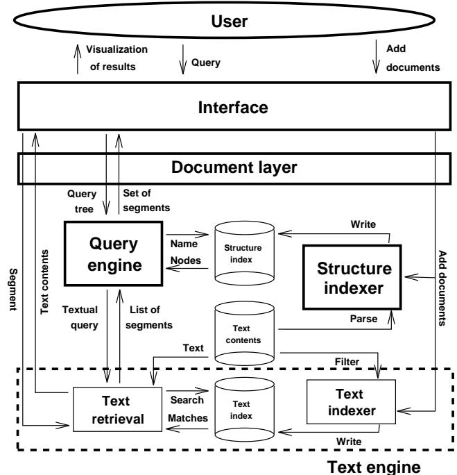
Figure 4: The architecture of a system following our model.
