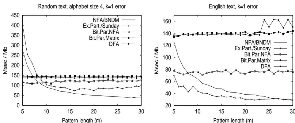
Fig. 20. Times in milliseconds per megabyte, for random and English and  $k = 1$  error under edit distance.
