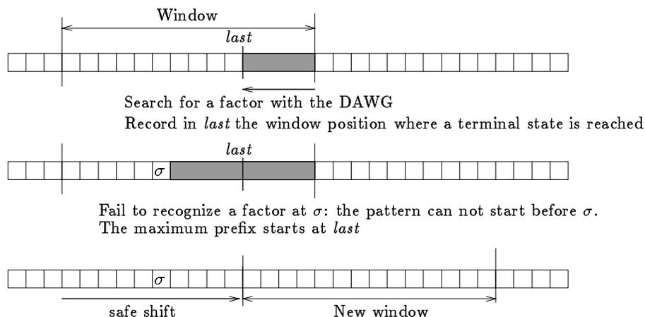
Fig. 3. Basic search with the suffix automaton
