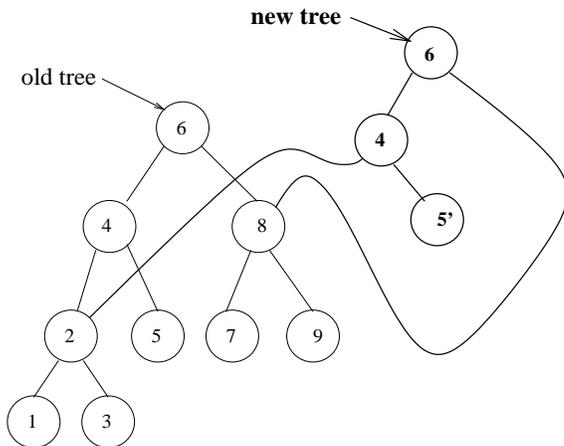
Figure 2: Changing node 5 to 5' in a read-only tree.
