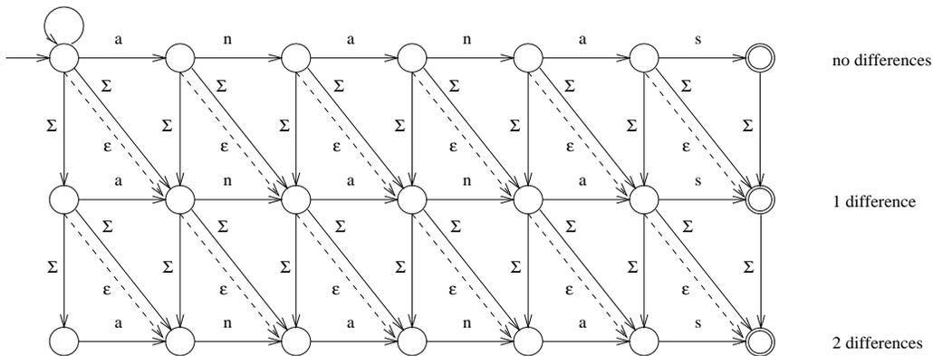
Figure 4: An NFA for approximate string matching of the pattern "ananas" with two differences.
