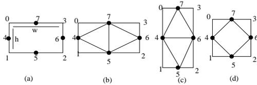
Figure 1. The tessellation of a 1-irregular rectangle with 4 Steiner points depends on the edge length ratio
