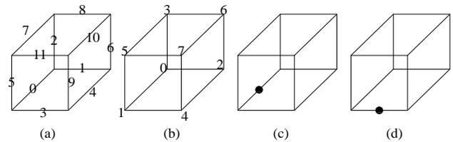
Figure 4. (a) Cuboid edge numeration, (b) cuboid vertex numeration, (c) one split edge pattern type, and (d) one split edge 1-irregular cuboid
