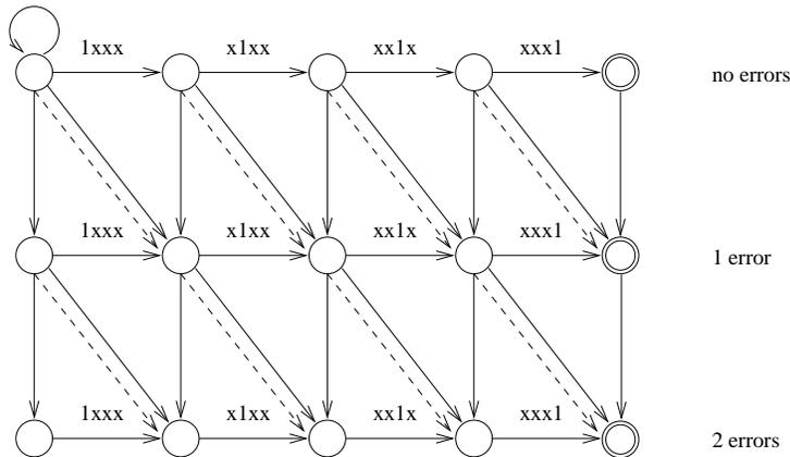
Figure 4: A nondeterministic automaton for approximate phrase searching (4 words, 2 errors) in the compressed text. Dashed transitions flow without consuming any text input. The other unlabeled transitions accept any bit mask.
