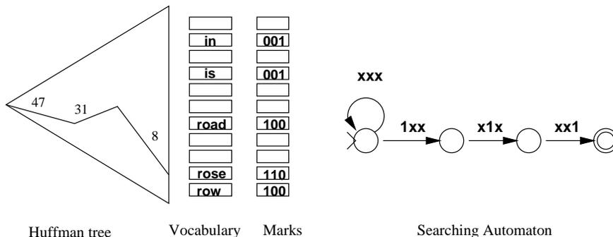
Figure 3: General searching scheme for the phrase "ro\* rose is" allowing 1 error. The x in the automaton stands for 0 or 1.
