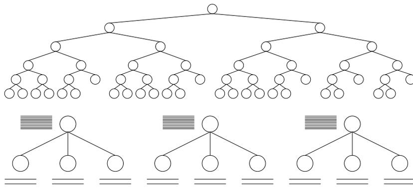
**Fig. 8.** Top: basic pattern hierarchy for 27 patterns. Bottom: pattern hierarchy with bit-parallel counters (27 patterns).
