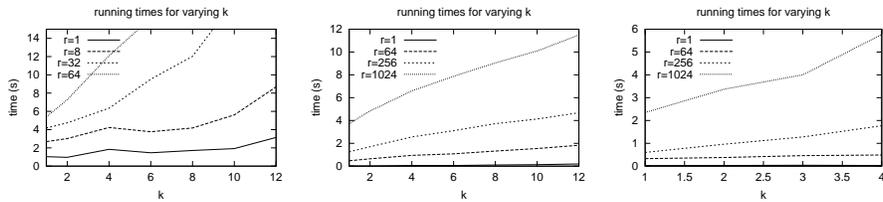
**Fig. 13.** Search times in seconds for exact pattern partitioning algorithm, for  $\sigma = 4$  (DNA),  $\sigma = 20$  (protein), and  $\sigma = 64$  (ASCII) alphabets.
