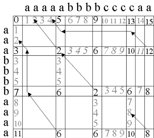
Figure 7: Evaluating the LCS between strings A = aaabbbbbaaaa and B = aaaaabbbbccccaa using the algorithm in Figure 6. The gray values denote the bridges, thus these values are not explicitly computed, but they can be deduced from the corner values.
