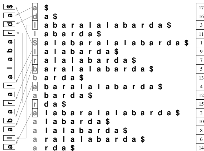
Fig. 6. The list of suffixes of S = \text{alabaralabarda}\$ in increasing lexicographic order. The sequence of preceding symbols (in gray) forms the BWT of S , S^{bwt} = \text{adll\$lrbbaaraaaa} . The run heads are boxed. To their left, we show how they are mapped to S and become the explicit symbols of the induced bidirectional macro scheme, using the same conventions of Figure 2. On the right we show the suffix array of S .
